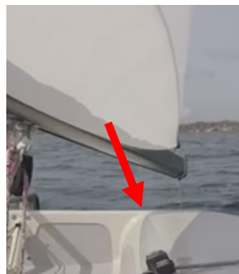
On flat water, I would never pull the traveller more than the area shown by the arrow
