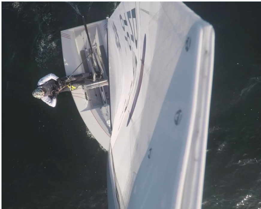
Medium winds - inhaul slacked about 1-2 cm to close the lowest part of the sail to gain power
